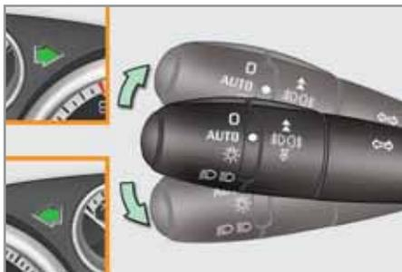
Raise or lower the lighting stalk passing the point of resistance; the corresponding direction indicators will flash until the stalk is moved from this position.
