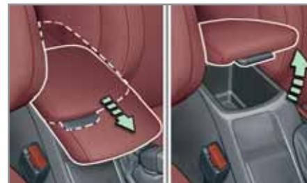
For your comfort, the height and the longitudinal position of the front armrest can be adjusted.
