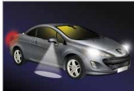
In the same way, the passenger compartment lighting, such as the courtesy lamps, the door sill lamps and the footwell lamps, comes on.
