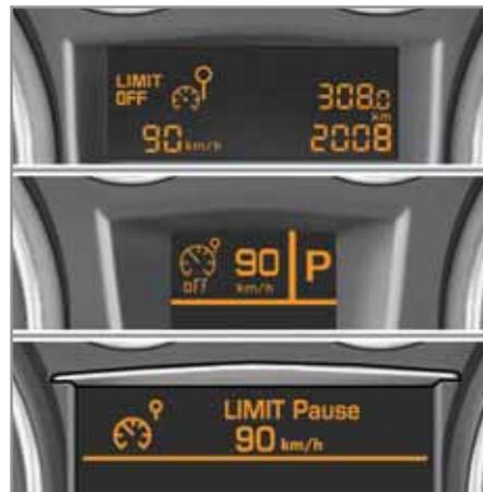
The cruise control or speed limiter mode appears on the instrument panel when it is selected.
