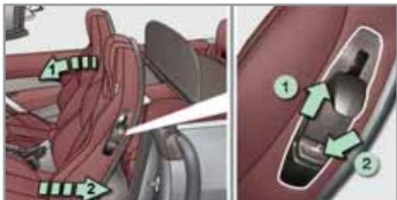
1. Control for release of the seat back and automatic forward movement of the seat.
