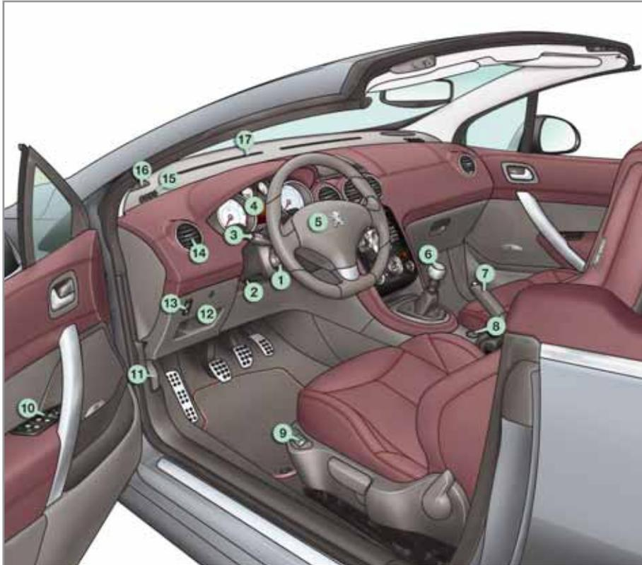
1. Cruise control/speed limiter switches.
