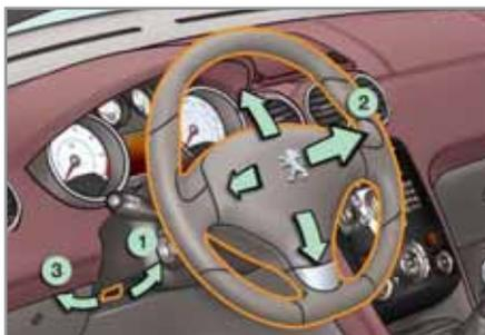
1. Release the adjustment mechanism.
